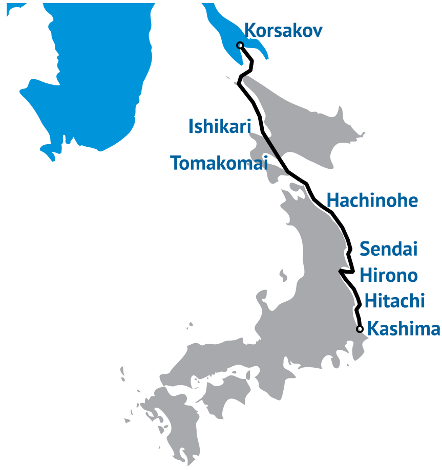
Figure 1. Proposed Subsea Pipeline Route*
